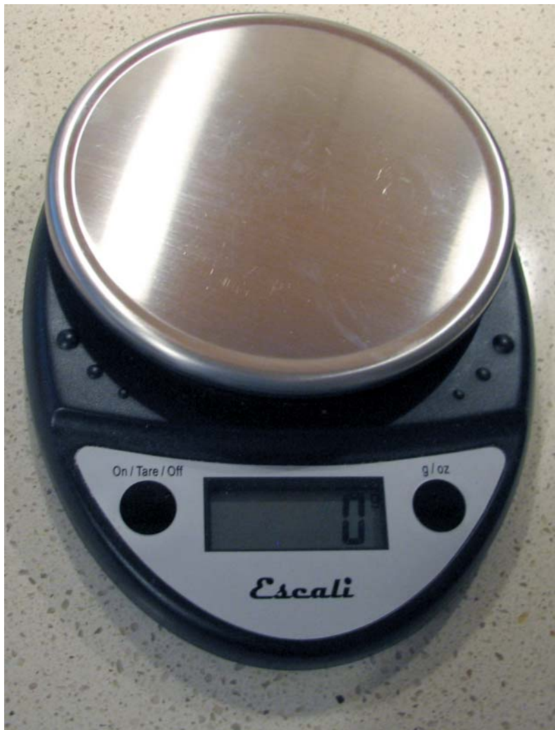
Figure 1.2.1: Modern scale for measuring cooking ingredients in grams, with a tare function
