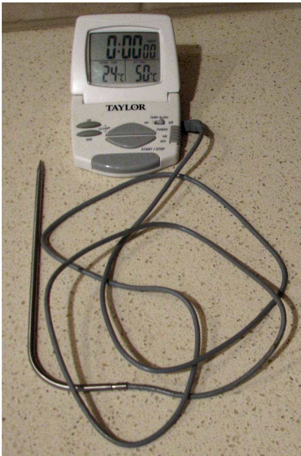
Figure 1.3.2: Digital thermometer with external probe for determining the internal temperature of food inside of an oven or broiler.
