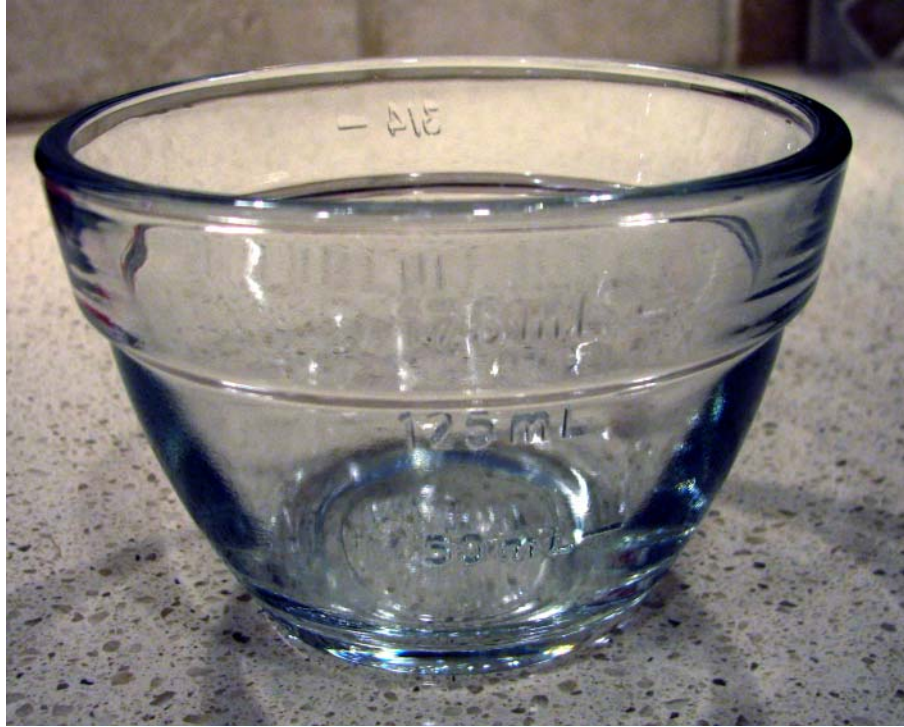
Figure 1.2.4: Ramekin with volume graduations of 50 mL, 125 mL and 175 mL. If one pours in 50 grams of water into the ramekin, the volume will be 50 mL.
