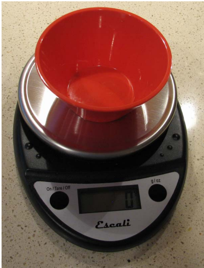
Figure 1.2.2: Small orange ramekin which is zeroed out with the tare button and ready to measure the quantity of an ingredient in a recipe.
