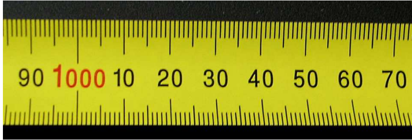
Figure 11.1: The 990 mm to 1070 mm section of a mm only Australian tape measure used in building construction.
