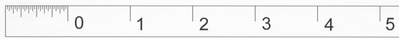
Figure 11.7: Ruler to illustrate the use of the first and last inch of US fractional rulers.
