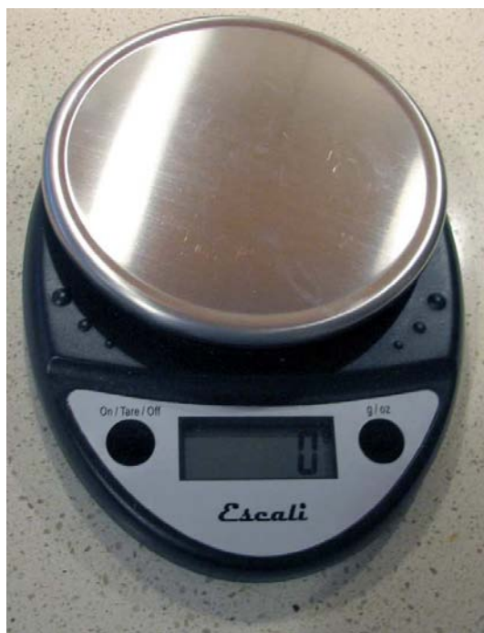
Figure 1.1: Modern scale for measuring cooking ingredients in grams, with a tare function
