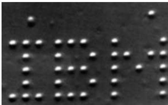
Figure 13.1: Image of the first set of letters written with individual atoms. The letters are 5 nanometers in height. Each dot is a single Xenon atom. (Courtesy of IBM Archives)
